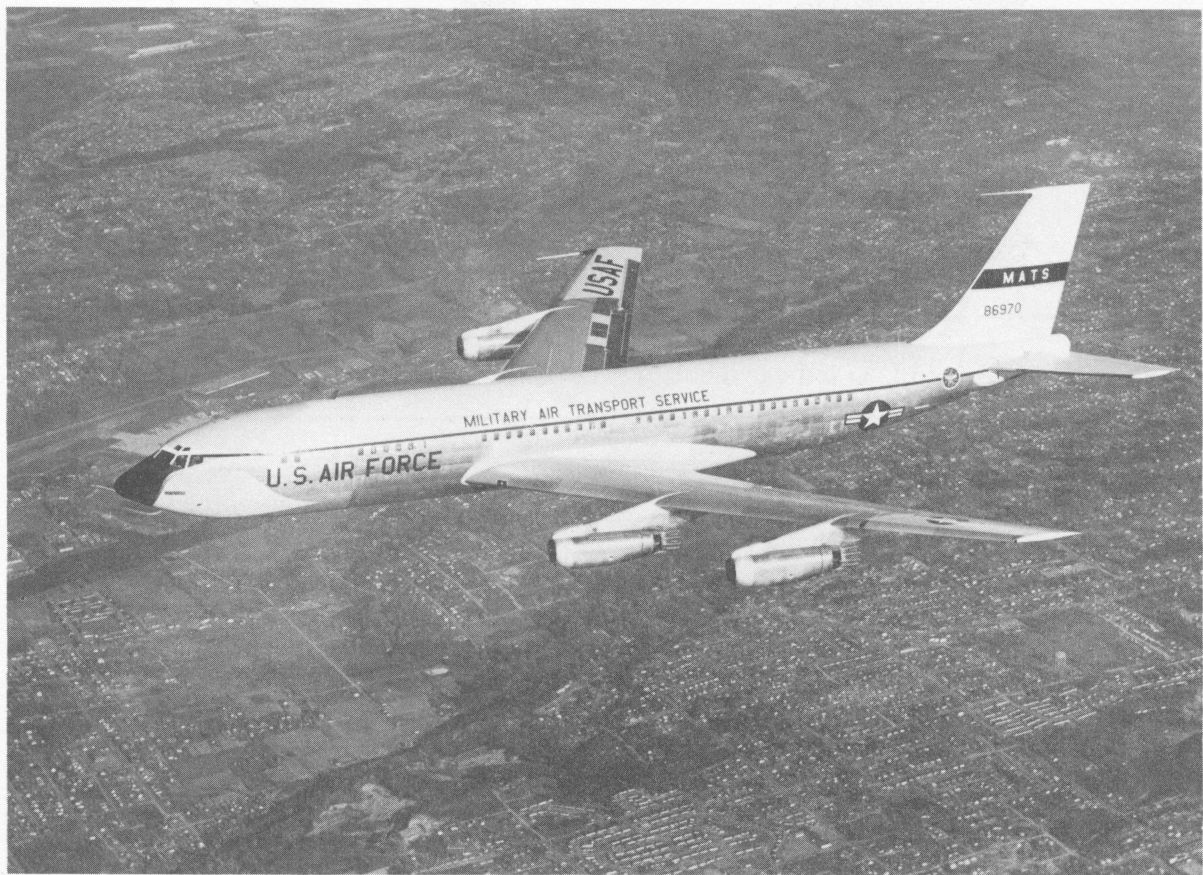
THE VC-137A SPECIAL PURPOSE JET TRANSPORT is being built by Boeing for the Military Air Transport Service. It has a non-stop range of 3500 miles and includes the latest communications facilities for en route work by government and military officials.
